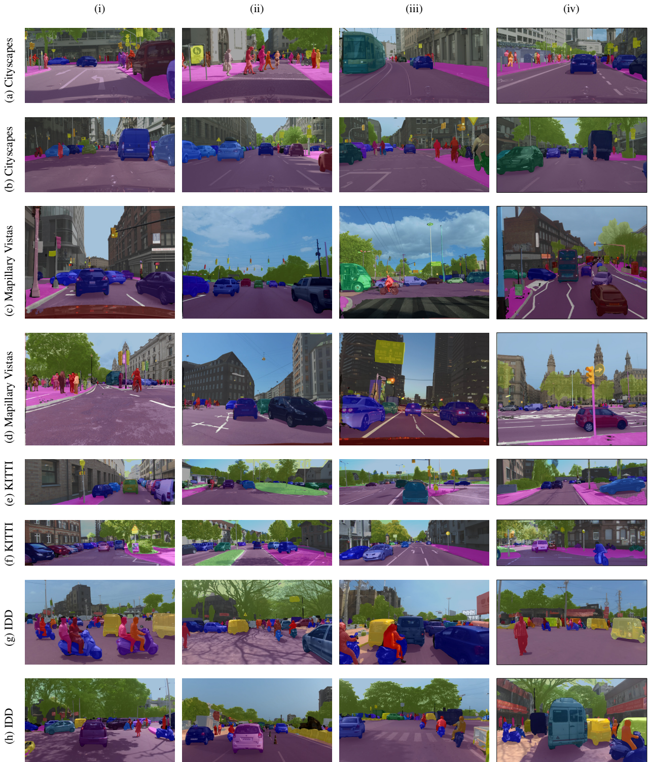
Figure 7 Visual panoptic segmentation results of our proposed EfficientPS model on each of the challenging urban scene understanding datasets that we benchmark on which in total encompasses scenes from over 50 countries. These examples show complex urban scenarios with numerous object instances in multiple scales and with partial occlusion. These scenes also show diverse lighting conditions from dawn to dusk as well as seasonal changes.
